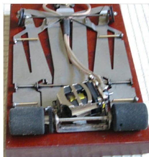
Note;- When fitting S16 motors to this chassis, the Proslot S16d and the majority of other makes will fit inside the motor box with careful alignment. A special centre section with an "unfolded" can end to the motor bracket is available for older types of set up where the motor may be mounted on top of the chassis.
