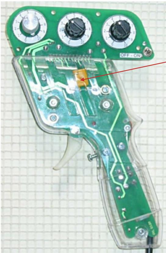
This is the brake resettable fuse. This is the more modern type, earlier controllers have a metal strip type fuse which is more likely to be sensitive to resistance gains. A replacement for this is;- multifuse BOURNS MF-R185 , available from RS or Farnell.
