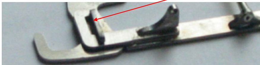
Solder Pin Tube mounts and Pin tube in place.
