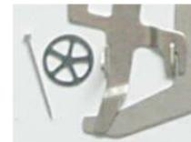
Fit lead wire clips and braids and solder on lead wires. Slip wires through the lead wire clip on the centre section of the chassis and connect to the motor.
