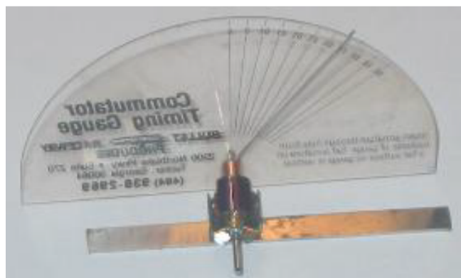
Checking the commutator advance using a timing protractor.
