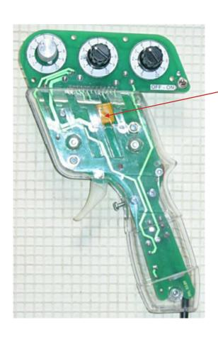
This is the brake resetable fuse. This is the more modern type, earlier controllers have a metal strip type fuse which is more likely to be sensitive to resistance gains. A replacement for this is;-multifuse BOURNS MF-R185, available from RS or Farnell.
