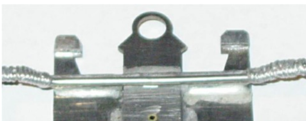
Polish underside leading edge of pan prior to installation. Add a small "skid" made from brass shim (braid clip) to front T bar and radius/polish.
