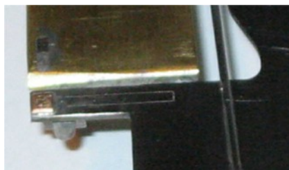
Polish underside leading edge of pan prior to installation. Add a small "skid" made from brass shim (braid clip) to front T bar and radius/polish.
